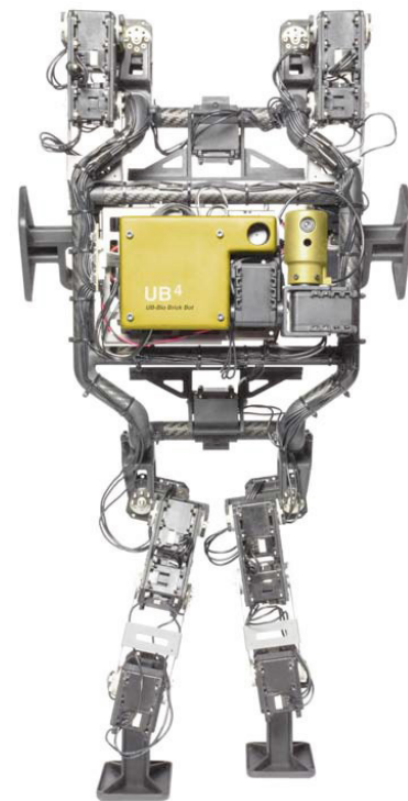
Figure 7: (Left) Two fully functional ABS 3d printed and titanium-sintered robot prototypes shown in stowed positions. (Right) A medium-scale humanoid mason uses an on-board video camera to navigate space and track objects in the environment.
